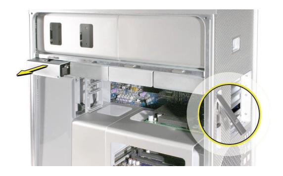
4. Remove the four screws that mount the drive to the carrier and remove the drive from the carrier.
